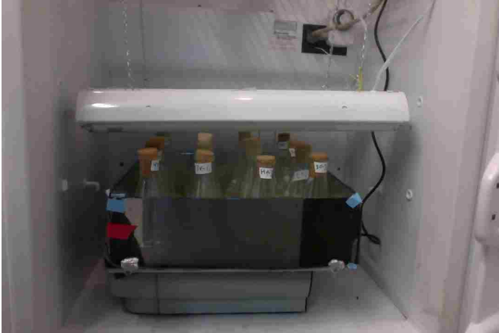
Figure 2. 3: Flask shaker table setup in temperature-controlled chamber.
